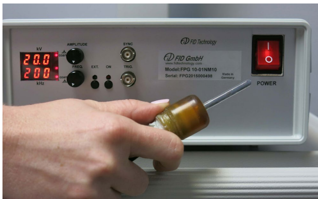
FIGURE 1 Cold atmospheric plasma device used for wart treatment. Custom made cold atmospheric pressure plasma device with hand-held electrode and pulse generator
