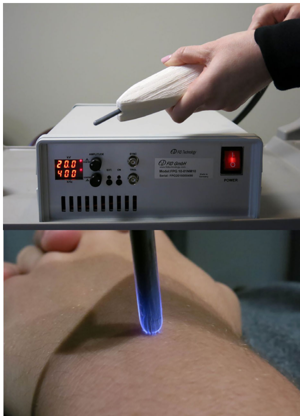
Figure 2 Floating-electrode DBD plasma. Top panel: pulse generator and hand-held electrode. Bottom panel: Plasma is being generated using the electrode tip. The electrode connected to the pulse generator must be kept near the treated surface. Either the tip or the side of the electrode can be used, but plasma will only form where the gap between the electrode and the target surface does not exceed 1 mm. The device pictured is an experimental prototype described previously by Friedman et al. 3
