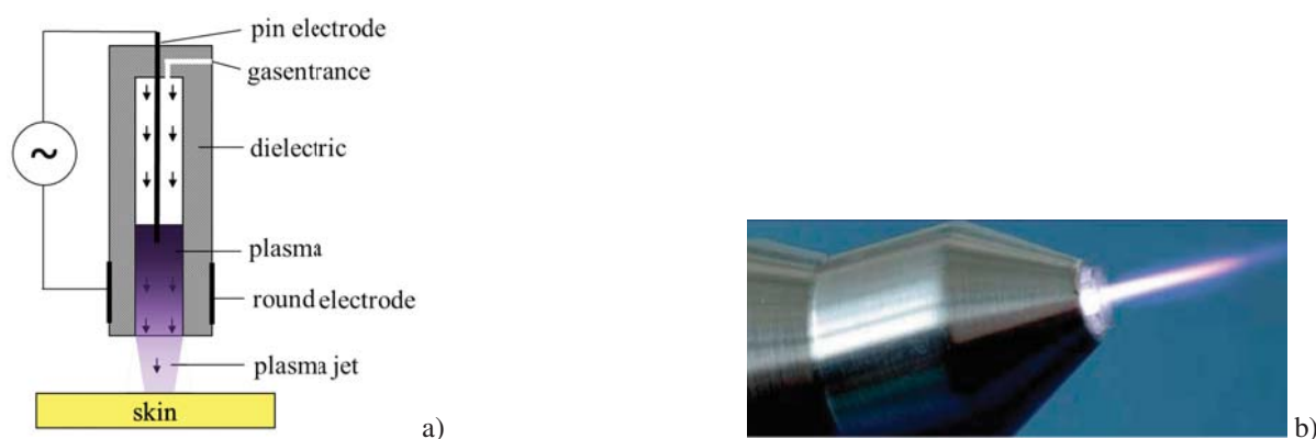
Fig. 1 One possible design of an indirect plasma source is schematically shown in (a) and a concrete device, the kinpen MED, is exemplified in (b).
